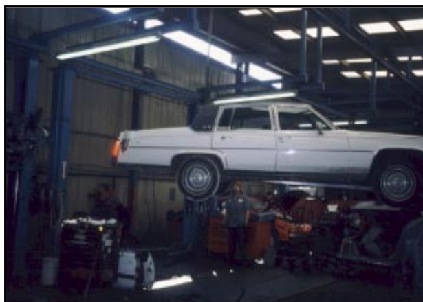
At this salvage yard, vehicles undergo fluid removal in an indoor area. The impervious floor helps contain any spills.
