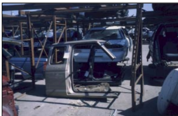
This salvage yard stores vehicles on a concrete surface until the fluids are removed.
